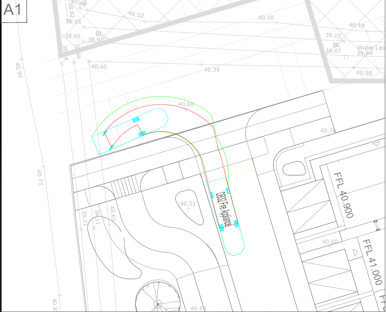
ZONE 1 SWEEP PATH ANALYSIS FOR FIRE TENDER SCALE 1:250
